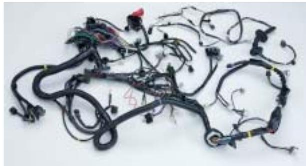
Wiring harnesses must be removed at an early stage of dismantling.
