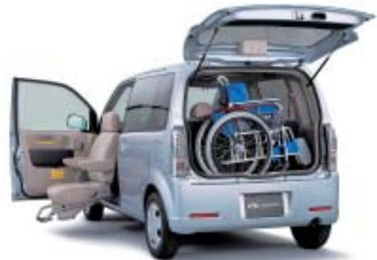
"eK Wagon" vehicle equipped with a movable passenger seat
